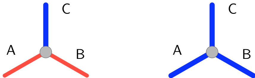
(a) AND vertex. Edge C may be directed outward if and only if edges A and B are both directed inward.
